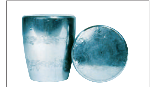
Photo 3-6 Part: Convex rollers of Photo 3-5 Symptom: Scoring on the roller end face Cause: Debris, which is caught in surface, and excessive axial loading
