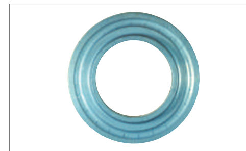
Photo 11-3 Part: Outer ring of a thrust ball bearing Symptom: False brinelling of raceway surface at ball pitch Cause: Repeated vibration with a small oscillating angle
