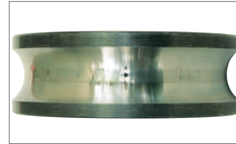
Photo 11-1 Part: Inner ring of a deep groove ball bearing Symptom: False brinelling occurs on the raceway Cause: Vibration from an external source while stationary
