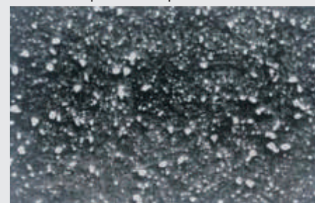
Distribution of carbides and carbonitrides in a Super-TF bearing. (X4000 magnification)
