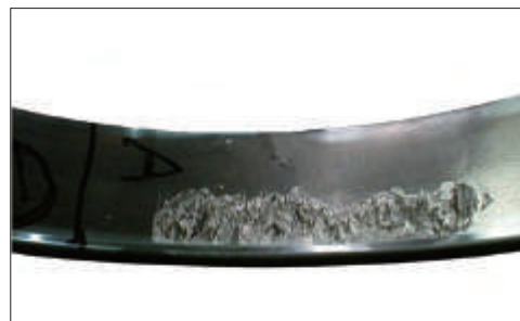
Photo 1-10 Part: Enlargement of raceway surface in Photo 1-9 Symptom: Flaking of one-side of the raceway Cause: Excessive pressure due to be misalignment
