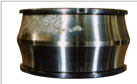
Photo 1-7 Part: Inner ring of a spherical roller bearing Symptom: Flaking of only one row of raceway Cause: Poor lubrication
