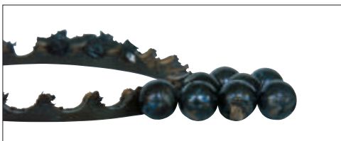
Photo 12-5 Part: Balls and cage of Photo 12-3 Symptom: Cage is damaged by melting, balls become discolored and melted Cause: Excessive preload
