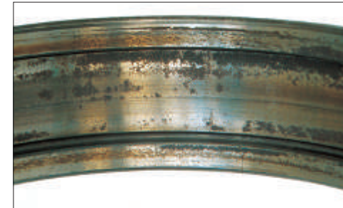
Photo 15-1 Part: Outer ring of a cylindrical roller bearing Symptom: Rust on the rib face and raceway surface Cause: Poor lubrication due to water entry
