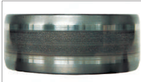
Photo 14-3 Part: Inner ring of a cylindrical roller bearing Symptom: Belt pattern of electrical corrosion accompanied by pits on the raceway surface
