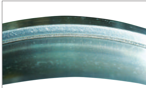
Photo 3-1 Part: Inner ring of a spherical roller bearing Symptom: Scoring on large rib face of inner ring Cause: Roller slipping due to sudden acceleration and deceleration
