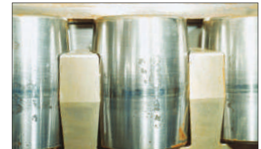
Photo 15-4 Part: Rollers of a spherical roller bearing Symptom: Pit-shaped rust on rolling contact surface. Corroded portions. Cause: Moisture condensation during storage
