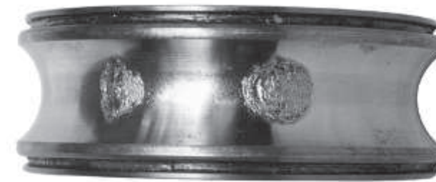
Fig. 4.1 Example of Flaking
