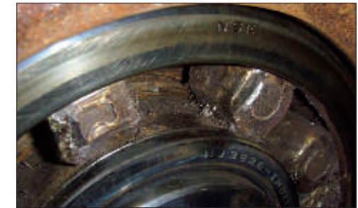
Photo 12-7 Part: Cylindrical roller bearing Symptom: Seizure occurs on ring raceway surface and roller Cause: Excessively small internal clearance causes heat generation by sliding of the inner ring and rollers under high speed and light load
