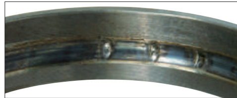
Photo 12-4 Part: Outer ring in Photo 12-3 Symptom: Raceway discoloration, melting occurs at ball pitch intervals Cause: Excessive preload
