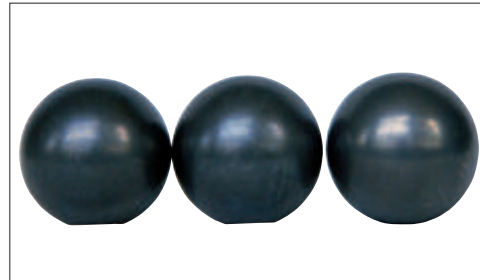
Photo 14-4 Part: Balls of a groove ball bearing Symptom: Electrical corrosion has a dark color that covers the entire ball surface
