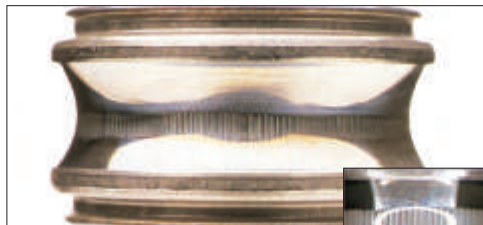
Photo 14-5 Part: Inner ring of a deep groove ball bearing Symptom: Fluting occurs on the raceway surface (High frequency)
