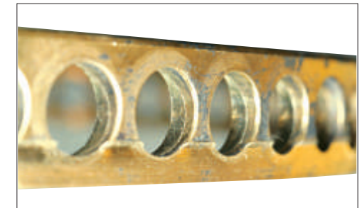
Photo 7-2 Part: Cage of an angular contact ball bearing Symptom: Stepped wear on the outside surface and pocket surface of a machined high-tension brass cage
