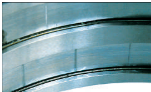
Photo 10-3 Part: Outer ring of a double-row cylindrical roller bearing Symptom: Fretting occurs on the raceway surface at roller pitch intervals
