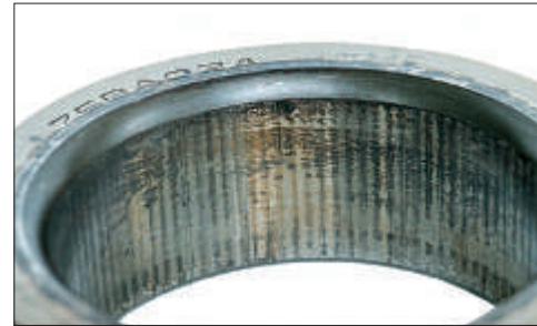
Photo 10-2 Part: Inner ring of an angular contact ball bearing Symptom: Notable fretting occurs over entire circumference of bore surface Cause: Insufficient interference fit
