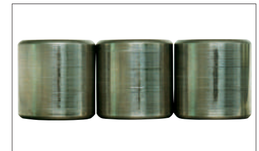
Photo 11-4 Part: Rollers of a cylindrical roller bearing Symptom: False brinelling occurs on rolling surface Cause: Vibration from an external source while stationary
