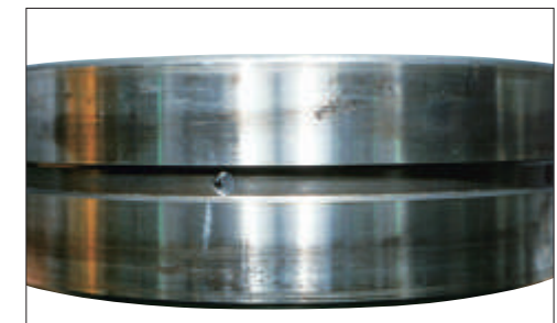
Photo 13-2 Part: Outer ring of a spherical roller bearing Symptom: Creep occurs over entire circumference of outside surface Cause: Loose fit between outer ring and housing
