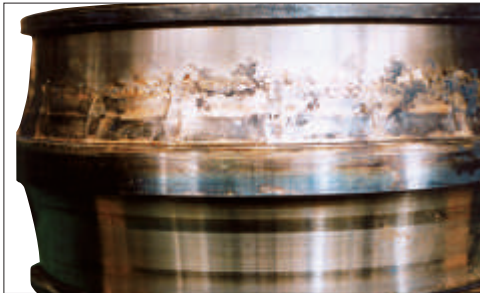
Photo 12-1 Part: Inner ring of a spherical roller bearing Symptom: Raceway is discolored and melted. Worn particles from the cage were rolled and attached to the raceway Cause: Insufficient lubrication
