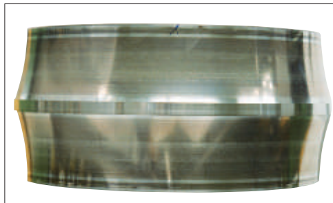
Photo 4-3 Part: Inner ring of a spherical roller bearing Symptom: Smearing occurs circumferentially on raceway surface Cause: Poor lubrication
