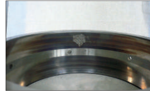
Photo 1-11 Part: Outer ring of a spherical roller bearing Symptom: Discoloration and flaking occur on outer ring raceway surface Cause: Poor lubrication under high temperatures
