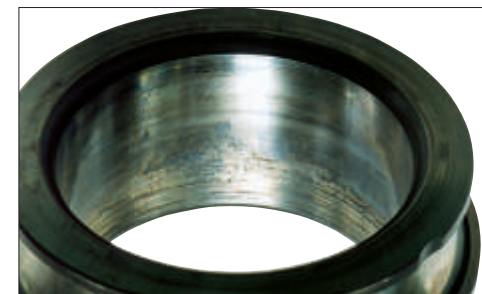
Photo 13-1 Part: Inner ring of a spherical roller bearing Symptom: Creep accompanied by scoring of bore surface Cause: Insufficient interference
