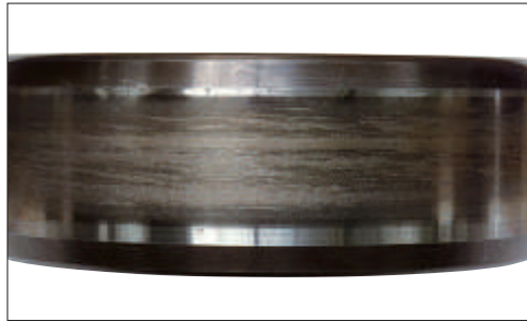
Photo 4-1 Part: Inner ring of a cylindrical roller bearing Symptom: Smearing occurs circumferentially on raceway surface Cause: Roller slipping due to excessive grease filling
