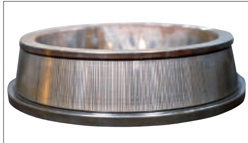
Photo 14-1 Part: Inner ring of a tapered roller bearing Symptom: Striped pattern of corrosion occurs on the raceway surface
