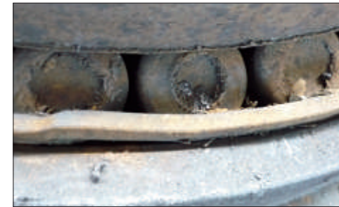
Photo 12-6 Part: Rollers of a large tapered roller bearing Symptom: Seizure occur at large end face of roller Cause: Poor lubrication and excessive axial load
