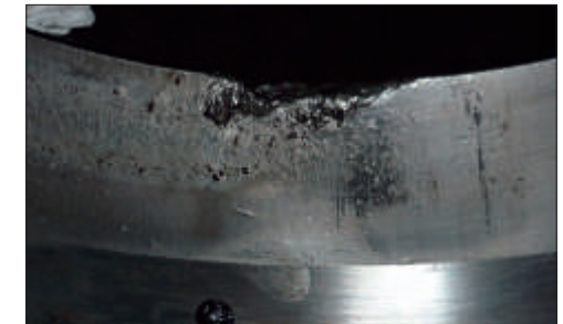
Photo 9-4 Part: Outer ring of a spherical roller bearing (enlargement) Symptom: Example of small flaking and wear combined on the raceway Cause: Insufficient oil film due to poor lubrication leads to wear (primary damage) that progresses to flaking (secondary damage)
