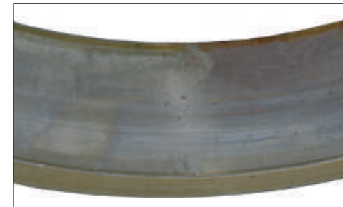
Photo 9-5 Part: Outer ring of a tapered roller bearing Symptom: Wear occurs on outer ring raceway surface Cause: Insufficient oil film and wear due to poor lubrication
