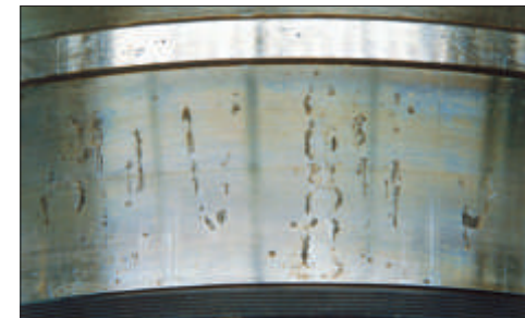
Photo 15-3 Part: Inner ring of a spherical roller bearing Symptom: Rust on raceway surface at roller pitch Cause: Entry of water into lubricant
