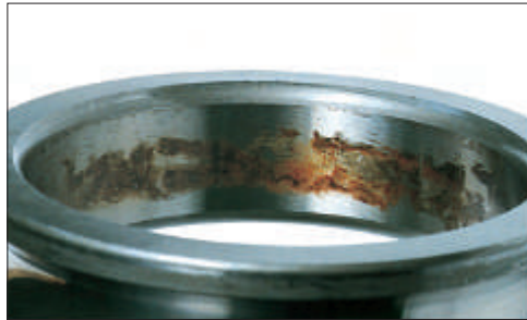
Photo 10-1 Part: Inner ring of a deep groove ball bearing Symptom: Fretting occurs on the bore surface Cause: Vibration
