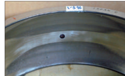
Photo 9-3 Part: Outer ring of a spherical roller bearing Symptom: Wear occurs on loaded side of raceway surface Cause: Low speed, heavy load and poor lubrication (No oil film)
