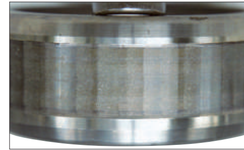
Photo 9-1 Part: Inner ring of a cylindrical roller bearing Symptom: Many pits occur due to electrical corrosion and wave-shaped wear on raceway surface Cause: Electrical corrosion
