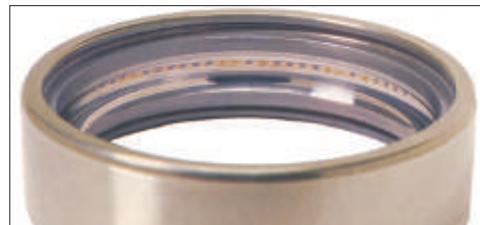
Photo 14-6 Part: Outer ring of a deep groove ball bearing Symptom: Fluting occurs on the raceway surface (High frequency)
