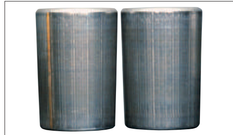
Photo 14-2 Part: Tapered rollers in Photo 14-1 Symptom: Striped pattern of corrosion occurs on the rolling surface
