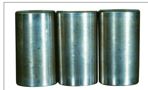
Photo 8-4 Part: Tapered rollers of Photo 8-3 Symptom: Small and large indentations occur over the rolling surface Cause: Debris caught in the surface
