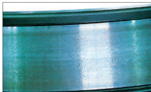
Photo 8-3 Part: Inner ring of a tapered roller bearing Symptom: Small and large indentations occur over entire raceway surface Cause: Debris caught in the surface
