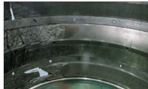
Photo 6-9 Part: Outer ring of four-row tapered roller bearing Symptom: Secondary damage after flaking occurs on outer ring raceway surface
