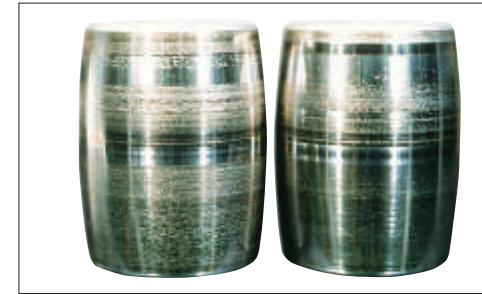
Photo 4-7 Part: Convex rollers of Photo 4-5 Symptom: Smearing occurs at the center of the rolling surface Cause: Poor lubrication
