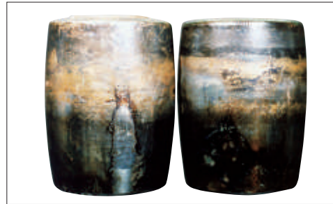
Photo 12-2 Part: Convex rollers of Photo 12-1 Symptom: Discoloration and melting of roller rolling surface, adhesion of worn particles from cage Cause: Insufficient lubrication
